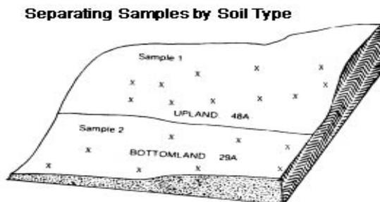
When sampling problem areas, collect separate samples from both the poor area and the good area to use as a comparison. It would be advisable to run a complete test on a surface sample and a sample from a lower depth to provide additional information. Include a description of the problem when samples are submitted so that A&L agronomists may assist you in finding a solution.
